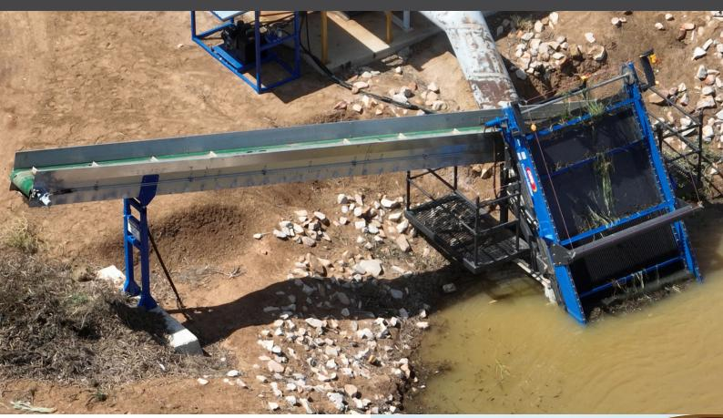
Keep your channels clear and pumps running efficiently with this innovative debris-filtering system.
